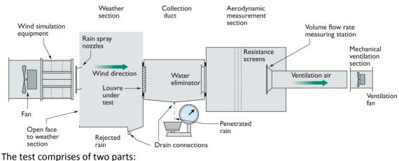
A schematic representation of the rig used during testing
