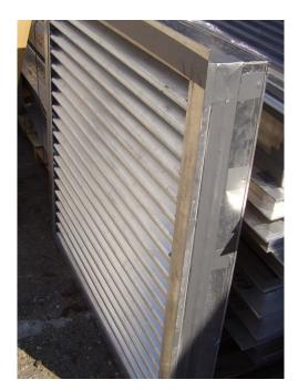
Note: Certificate 54763/1 Edition 1 described the louvre as having 2 banks of blades. The louvre has a single bank of blades, with a profile which extends almost the full depth of the unit. The test item information above has been amended. No other changes have been made.
