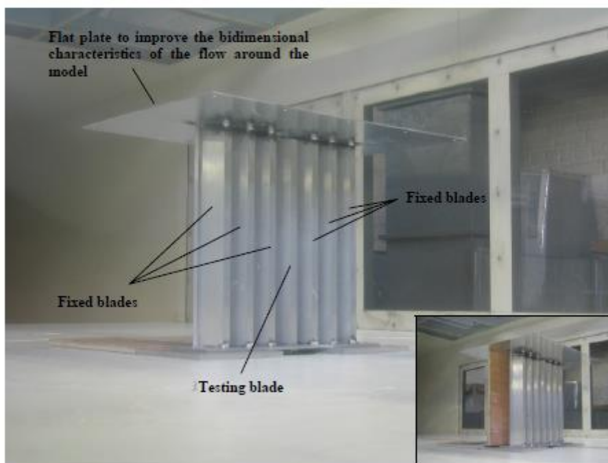
Figure 2.2. General arrangement in the wind tunnel of the model, and picture of a Linius® blades model (see table 2.1). In the down-right corner the wooden plate placed downstream the model to simulate the wall is shown.
